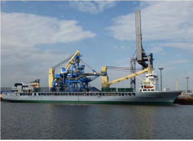
A purpose built heavy-lift ship designed for project cargoes.
