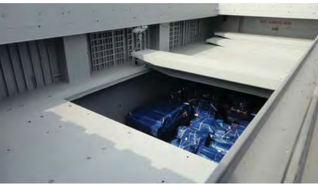
The tweendeck of a purpose built multi-purpose vessel.
